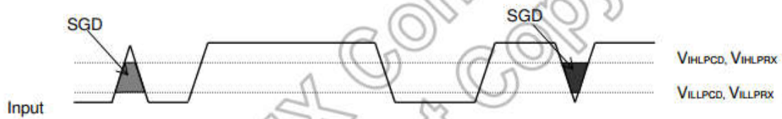
Figure 7.1: Input glitch rejections of low-power receivers
